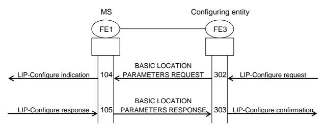
Figure 5.4: MS receiving basic parameters and sending response to it
