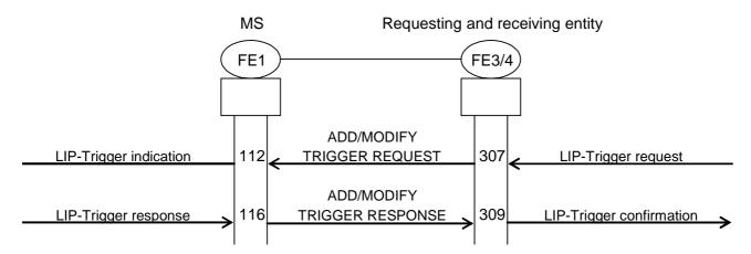
Figure 5.11: MS receiving trigger definitions and rejecting triggers
